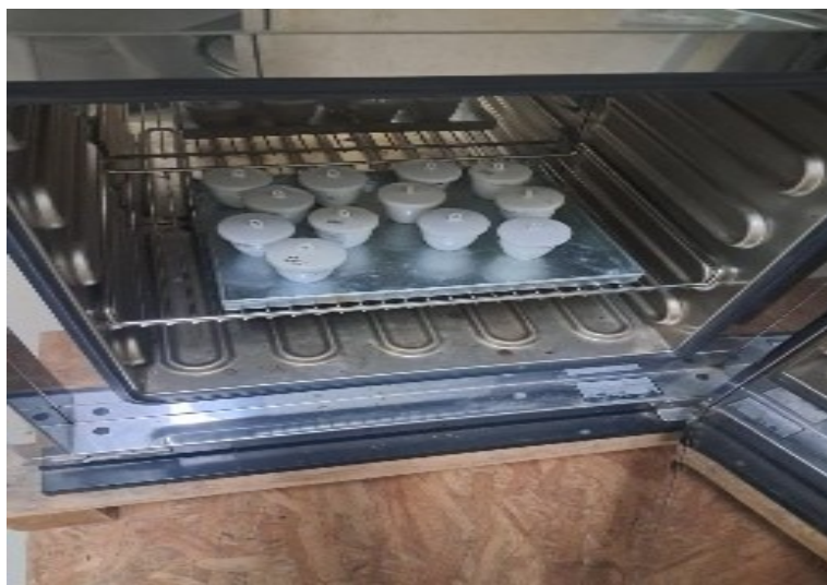
Figure 1. Testing the moisture content of yogurt with the addition of lamota extract
